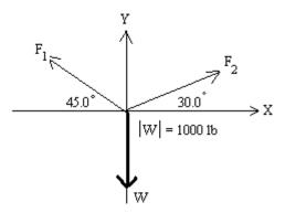
$F_1$  = the tension in left cable  $F_2$  = the tension in right cable
