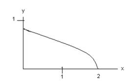
B) Notice the graph is at a max (y-value) when x=0, which is when the pendulum is in mid-swing. At this time the velocity of the pendulum is at a maximum. When the pendulum gets to then end of a swing the velocity goes to 0.
