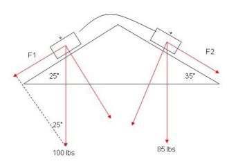
Like figure 10 on page 600, the figure above shows the blocks broken into the respective forces. We are solving for the forces parallel to the ramp. The side with the most downward force (parallel to the ramp) will be the direction of travel.
