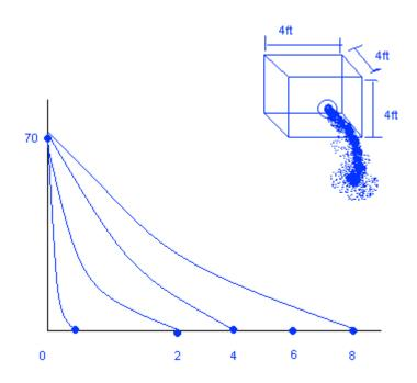
V(t) = volume of water in the tank t minutes after water begins to flow: =  $\frac{64}{c^2}(c-t)^2$  $0 \le t \le C$
